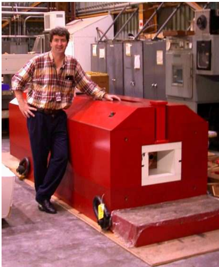
Figure 7.21: Close up of the TAN showing the cavity which will hold the ZDC.
