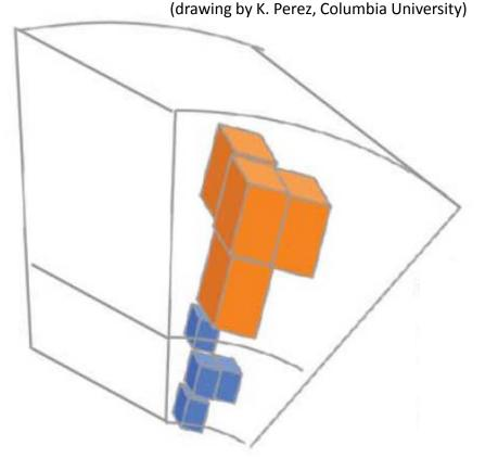
Topological cell cluster is a "blob" of energy dynamically located inside the calorimeter (even crossing sub-detector boundaries)
