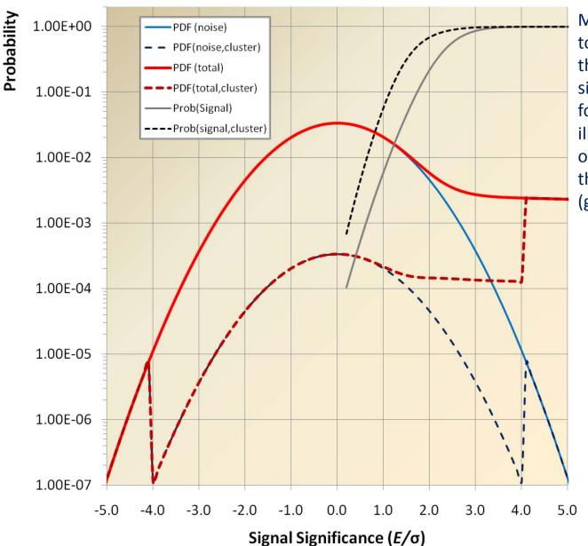
Modeled effect of topological clustering on the cell signal significance spectrum, for purposes of illustration here with only the primary (seed) threshold, no secondary (growth) threshold.
