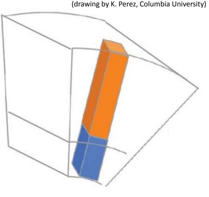
Unbiased calorimeter tower is a "slab" of energy in a regular pseudorapidity-azimuth grid (each tower covers the same area in these coordinates)
