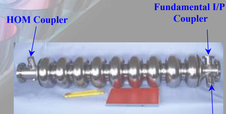
9-Cell Niobium Cavity Suitable for ILC
