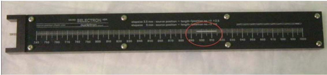
Figure 8 Source position ruler showing white plastic indicator (red circle).
