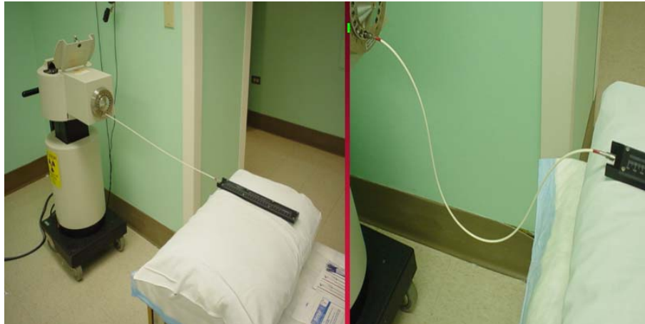
Figure 9 Source position accuracy test showing a well-aligned ruler, transfer tube, and afterloader (left) and a set-up with a large curvature.
