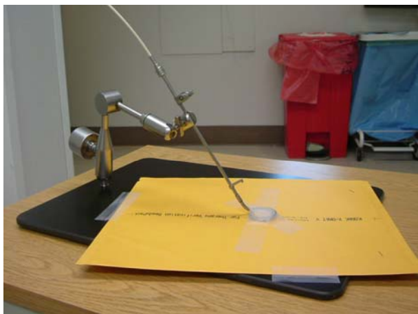
Figure 2 Photograph of a ring applicator secured to a base plate with film taped securely in place.
