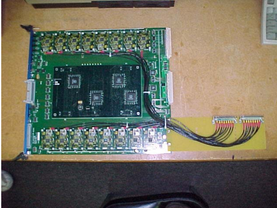
Figure 1. Photograph of the L1MU motherboard, MTC05 daughter card, and serial link receivers.
