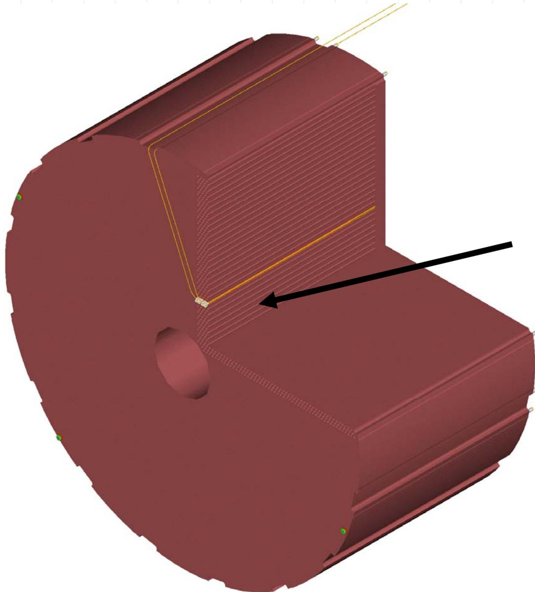
Ionization rate is worst near inner edge at  $|\eta| \sim 4.7$  at depth near EM shower max
