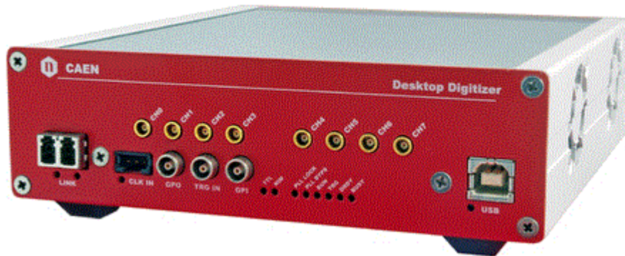
Fig. 13: CAEN digitizer. This module has 8 channels of 14 bit, 500 \text{ MHz} sampling rate ADCs, 512 \text{ MSamples/channel} memory, 50 \Omega input impedance, and a 250 \text{ MHz} bandwidth amplifier at the input which can switch between two gains.
