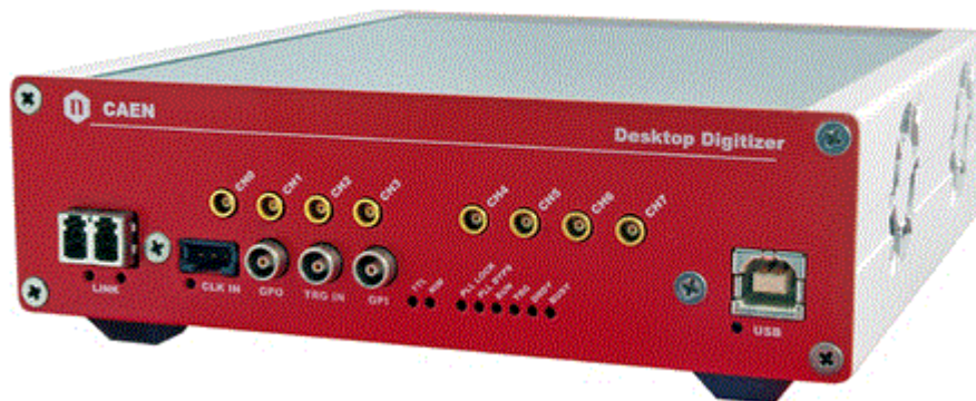
Fig. 13: CAEN digitizer with 8 channels of 14 bit, 500 MHz sampling rate, 512 MSamples/channel memory, 50\ \Omega input, 250 MHz bandwidth amplifier at the input which can switch between two gains.
