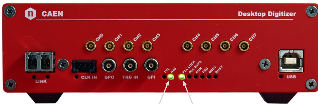
Fig. 12.1: Front panel LEDs status at power ON
