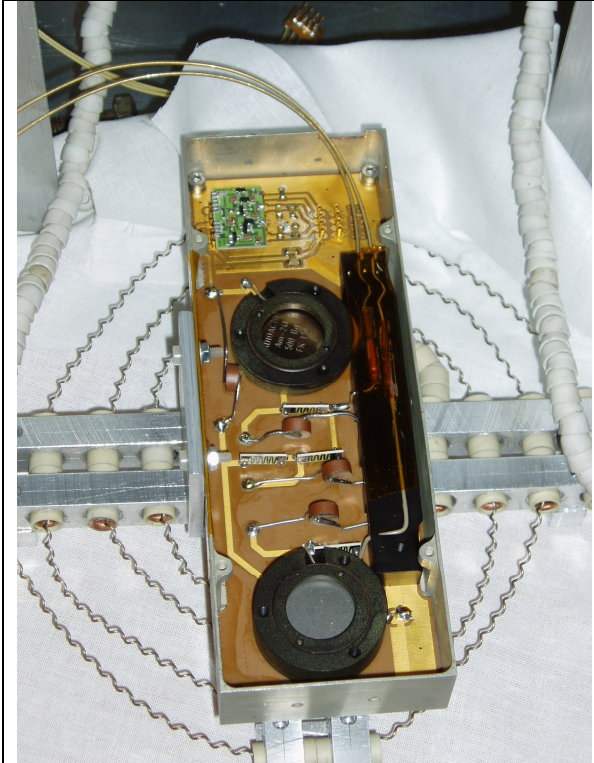
Purity monitor and new heating coil
