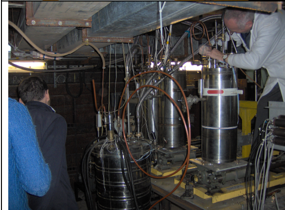
Cryostats in the beam area. Hooking up cooling and argon lines
