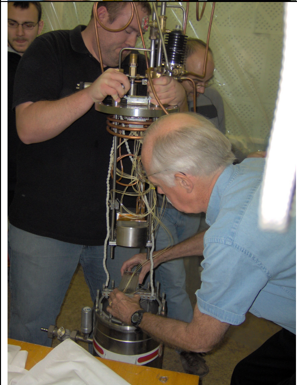
Reinstalling the FCalchik complete with new heater and purity monitor into the cryostat.
